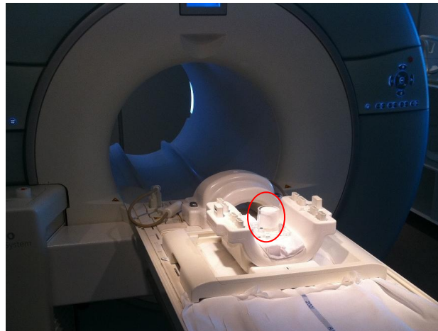
Fig.4 Heel pad phantom (marked by the red circle) placed inside the coil in the MRI scanner
