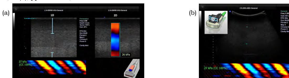
Figure 1: Current interface of the transient elastography on the SonixTouch ultrasound machine for both (a) linear transducer and (b) curvilinear transducer. The interface for both 1D and 2D modes for linear transducer are also displayed in (a).
