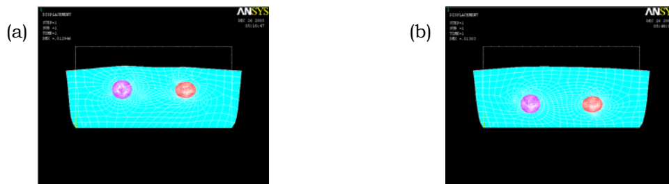
Figure 1: Results of computer simulation experiment. The size of numerical phantom (80 mm W x 40 mm H) of fat with elastic modulus of 18kPa was assumed [1]. Also assumed are circular mammary gland of the diameter of 10 mm (on the left side of the figures) with elastic modulus of 28 kPa and cancer of the diameter of 10mm (in the right) with elastic modulus of 106 kPa inside the fat. The assumed water pressure is 5 kPa. Poisson's ratio was assumed to be between 0.49 and 0.35 (in the above image it is 0.40). Elliptic deformation of mammary gland is evident, while that of cancer is not. In Figure 1(a), the depth of the centers of the circular lesions is 15 mm from the surface and in Figure 1(b), it is 25 mm. The height-to-width ratio of tissues was nearly independent of depth.
