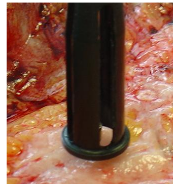
Figure 2: Demonstration of the Indentation Test Using the Hand-Held Probe on a Fresh Breast Tissue Sample.
