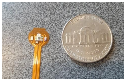
Left: New "smart" grasper prototype, with one of its flex PCBs separated (below); Right: One of the jaws, with the pulse oximetry LEDs and photodiodes, and the thermistor, next to a US 5 cent coin for scale
