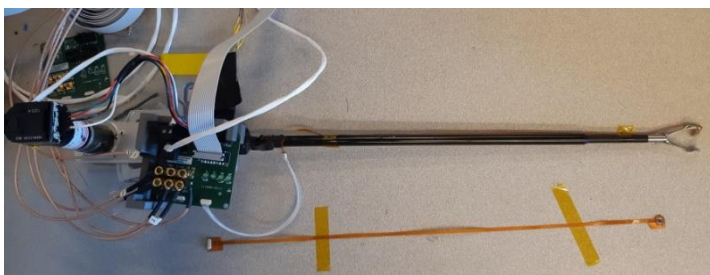
Left: New "smart" grasper prototype, with one of its flex PCBs separated (below); Right: One of the jaws, with the pulse oximetry LEDs and photodiodes, and the thermistor, next to a US 5 cent coin for scale
